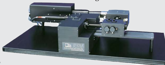
The RSM configured for fluorescence.
