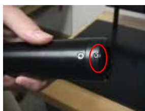
Loosen the set screw.
